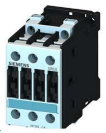
CONTACTOR, AC-3 4 KW/400 V, AC 220 V 50 HZ / 240 V 60 HZ, 3-POLE, SIZE S0, SCREW CONNECTION
